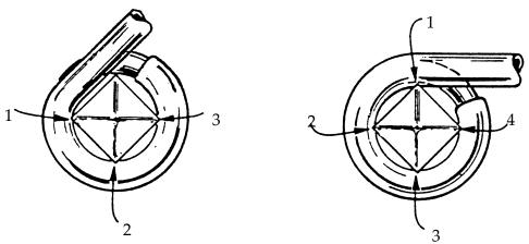
Shows either 3 or 4 corners of contact of insulation minimum  $^{3}\!\!/_{4}$  turn of insulated wire
