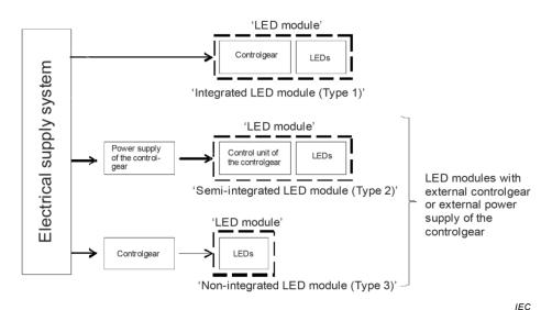
The power supply of the controlgear for semi-ballasted LED modules (Type 2) is an electronic device capable of controlling currents, voltage or power within design limits.
