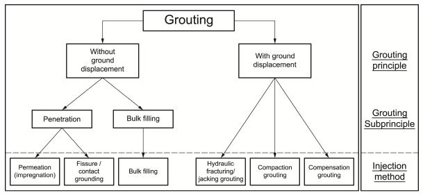
NOTE The term consolidation grouting is sometimes used to emphasize an improvement in the strength or deformation characteristics of a soil or rock mass, with the aim that it does not undergo any unacceptable deformation. The term compensation grouting is used when the objective of grouting is to concurrently compensate for ground loss.
