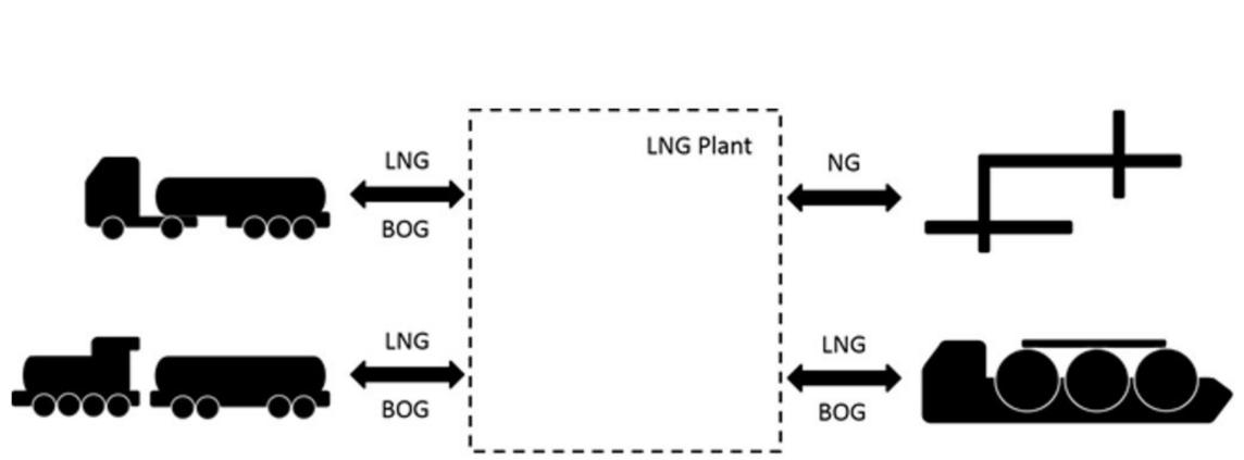
**Figure 1 — Boundary limits of onshore liquefied natural gas (LNG) installations**
