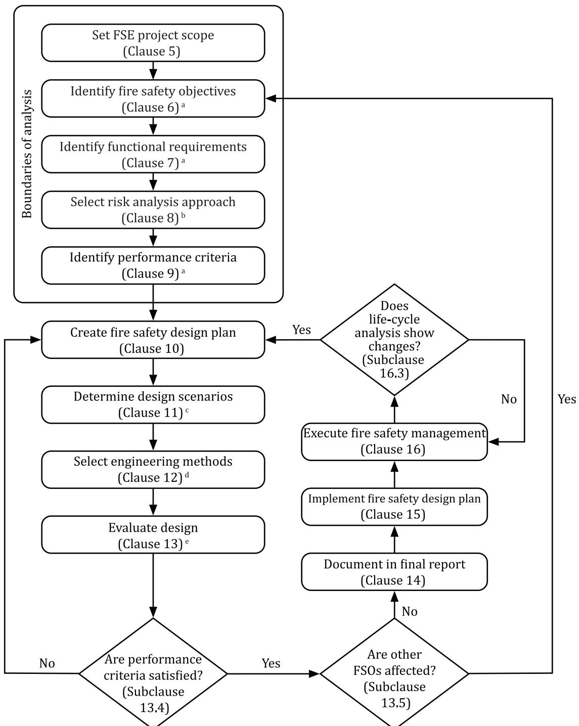
**Figure 1 — Flow chart of the fire safety engineering process**
